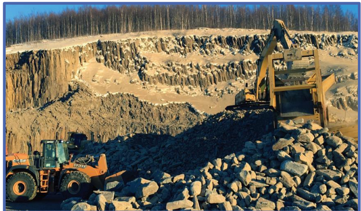
Mueller Mountain rock quarry was used for source of rock riprap for the levee.
