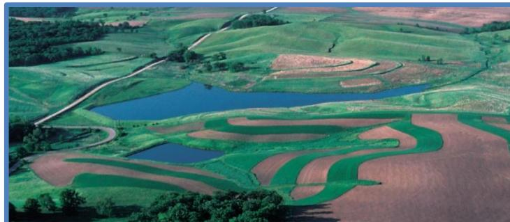
Conservation practices are a vital part of all watershed projects. Practices such as terraces, waterways, grass buffers and grass plantings were installed in this Tama County, Iowa watershed to prevent soil erosion and reduce sediment. Entrapment of sediment upstream from the dam increases the service life of the dam and its ability to provide flood control.
