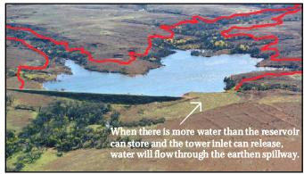
The red line on this photo indicates the extent that water can back up in the flood pool upstream before it starts flowing through the earthen spillway. This is where flood water is stored while it is slowly released through the principal spillway pipe.
